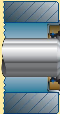
Figure 5: Use of a "TAY" design to prevent seal cocking
