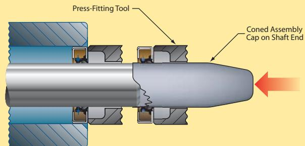
**Figure 9:** Use of cone as cap
