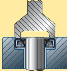
**Figure 7:** Tool designed to bottom the seal in a stepped housing
