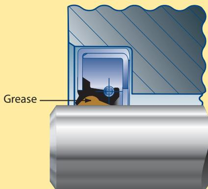
**Figure 3: Grease packing to provide seal and shaft lubrication**
