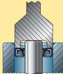
**Figure 8:** Tool designed to bottom out on the shaft face
