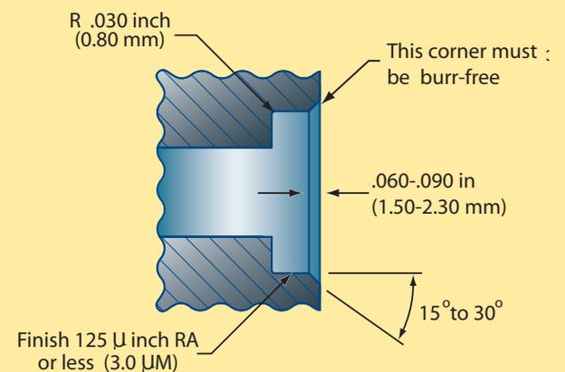
**Figure 1: Bore chamfer, radius, and surface finish recommendations**
