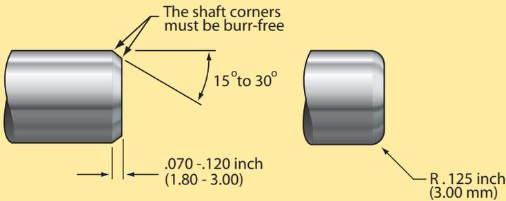
Figure 2: Shaft chamfer and radius recommendations
