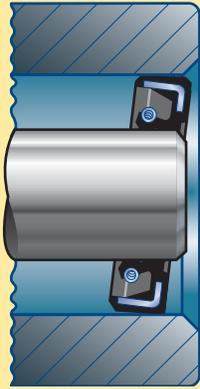
Figure 4: Misaligned (cocked) seal
