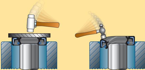
Figure 11: Use of a strike plate to prevent deformation
