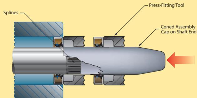
**Figure 10:** Use of cone as sleeve
