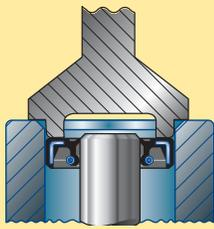
**Figure 6:** Tool designed to bottom out on the housing face
